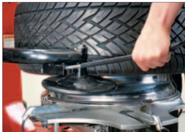
Bottom roller disc assists in re loosening tire beads and lifting the tire up the wheel barrel during demounting.
