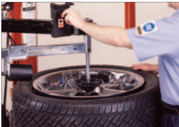
Pneumatic wheel press cones and extension arm simplify external alloy wheel clamping when servicing low-profile tires.
